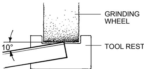
FIGURE 4--Grinding Side 1.
