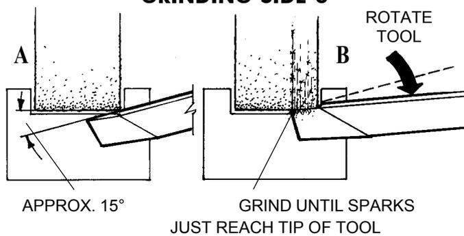
FIGURE 9--Grinding the "Hook" into side 3.
