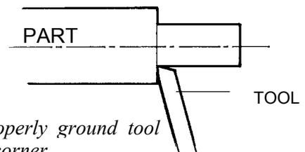
FIGURE 7--Properly ground tool cutting into a corner.
