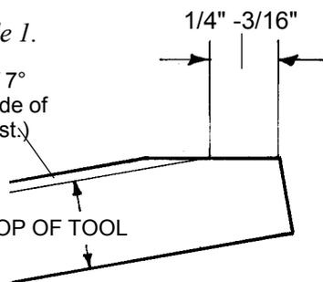
Move the blank back and forth across the face of the wheel until you have ground a 10° angle on approximately 3/16"
