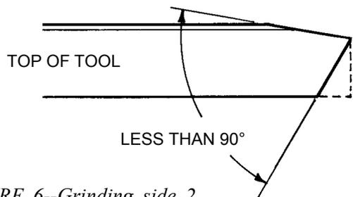
FIGURE 6--Grinding side 2.
