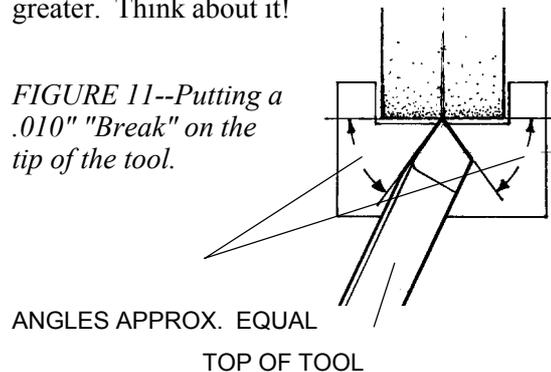
This means that if you set the tool flat on the tool rest the tool rest angle would have to be increased to get an even flat. This wouldn't be worth the effort, so the easy way is to free hand it. I always start by touching the heel of the tool first, and then change the angle until a slight flat is put on the tip. Of course, the angle you're holding it at has to be close when starting to get desired results.
