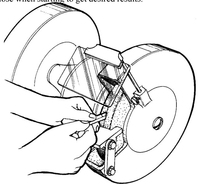
FIGURE 12--Handholding the tool to "Break" the point saves resetting the angle on the tool rest.
