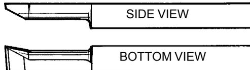
FIGURE 13--Typical Boring Tool.
