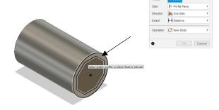
Enter the distance as a negative value to cut the part out. Confirm with enter and the area between polygon and circle will be removed.
