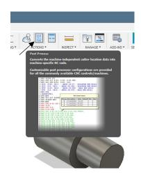
In the Post Process menu, select the location where the post processors have been stored to.
