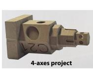
Complex turned parts with radius and tapered elements are difficult to produce on conventional lathes. This project demonstrates the advantages of computer-aided manufacturing.
